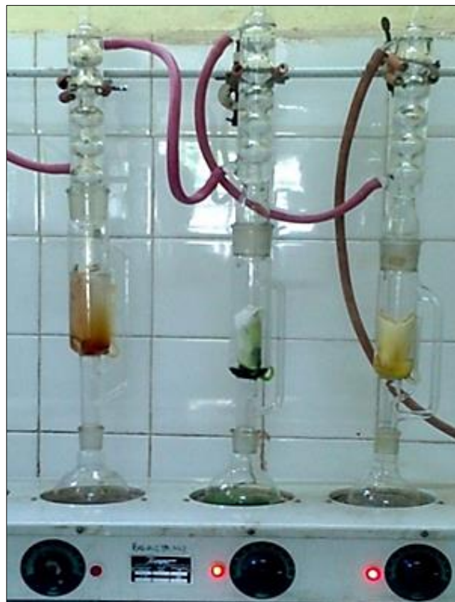
Fig 4: Soxhlet apparatus for extraction of phytochemicals
